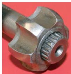
Machine down as shown to access snap ring
